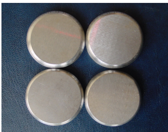
Fig.1. The mobile semi coupling made out of steel OLC 45
